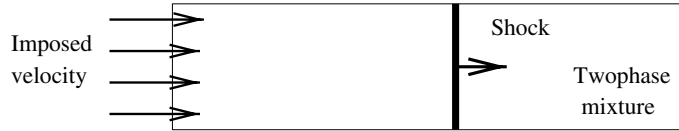
Fig. 8. Schematic representation of the two-phase impact problem.
